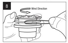
NOTICE: Failure to wind the line in the direction indicated will cause the bump head to operate incorrectly.
